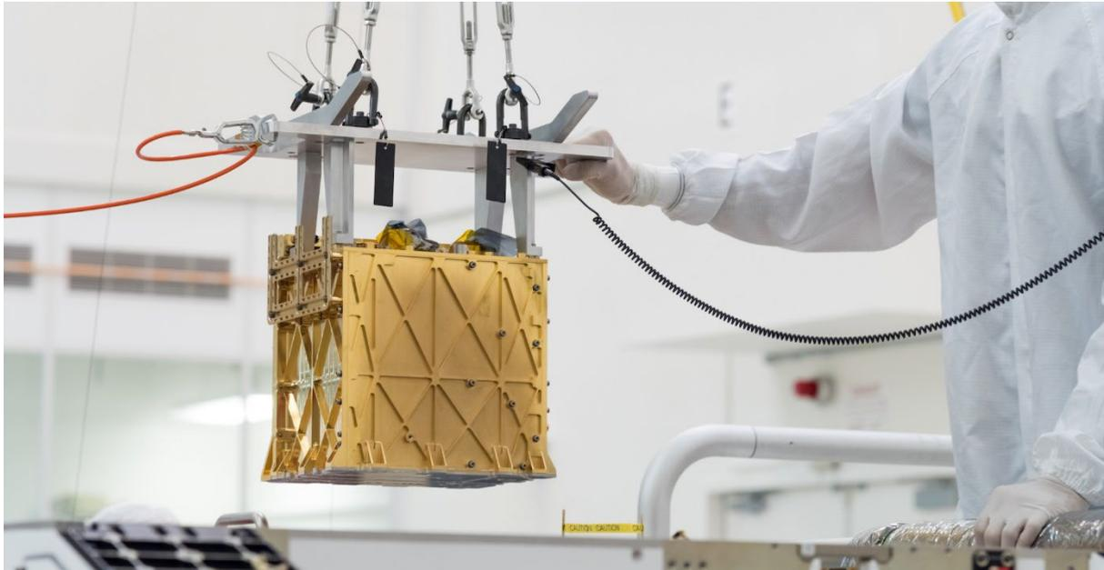
The Mars Oxygen In-Situ Resource Utilization Experiment (**MOXIE**) is an instrument on the **Perseverance Rover**. It makes **oxygen (O<sub>2</sub>)** out of **carbon dioxide (CO<sub>2</sub>)** gas in the Martian atmosphere.
