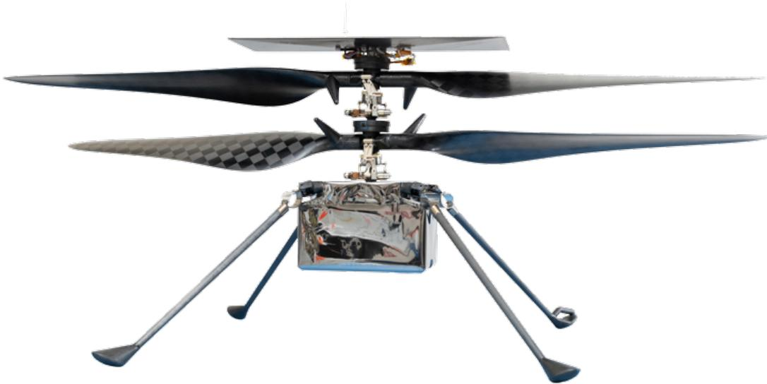
The **Ingenuity helicopter** is a **self-piloting drone** that came to Mars with the **Perseverance rover**. Its lightweight construction and long blades allow it to fly in the **thin Martian atmosphere**.
